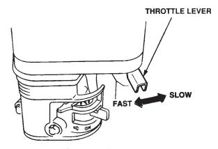
Figure 14. Throttle Lever
